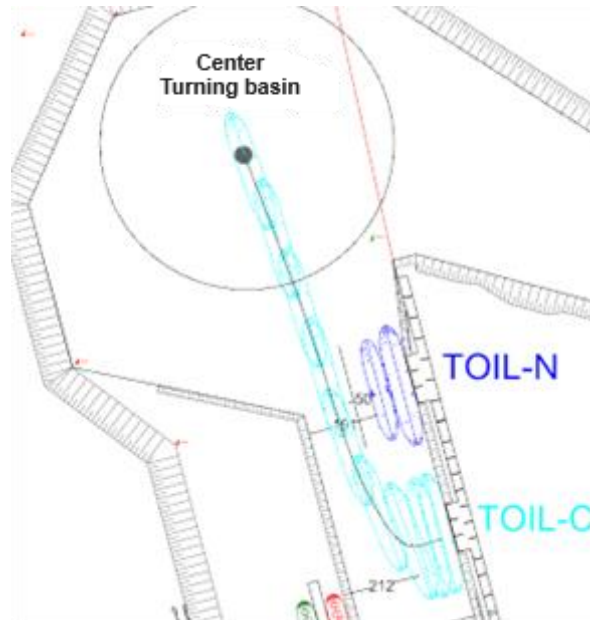
Figure 12 – Reference trajectories for berthing maneuver at TOil-C.
